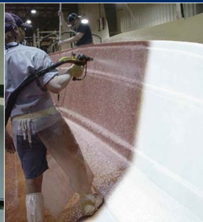
Sound Proofing & Protective Coating for Boat Inner Hulls
